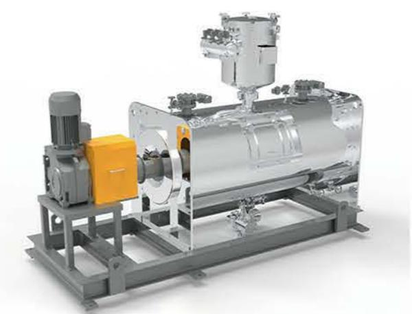
This equipment can be used for mixing of powder-powder, powder-minor liquid and low viscosity liquid. Typical applied for lithium battery cathode materials, precursor materials, real stone paint, feed, pesticide, plastic, etc. The size ranges from 0.5 cubic meters to 35 cubic meters.
